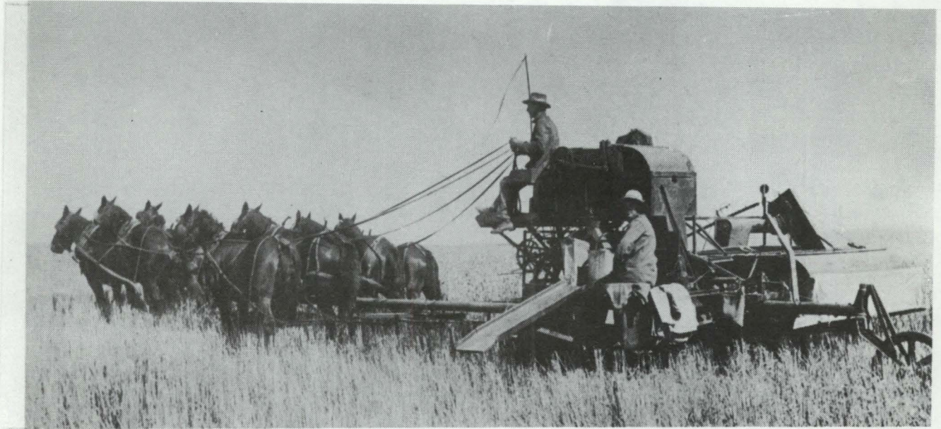
Pulling instead of pushing - Idaho harvester. Eight horses were pulling the 8-foot Idaho National Harvester originally constructed to be pushed. The beam used to push the combine was converted to a tongue. This was necessary for control of the direction of the machine.
