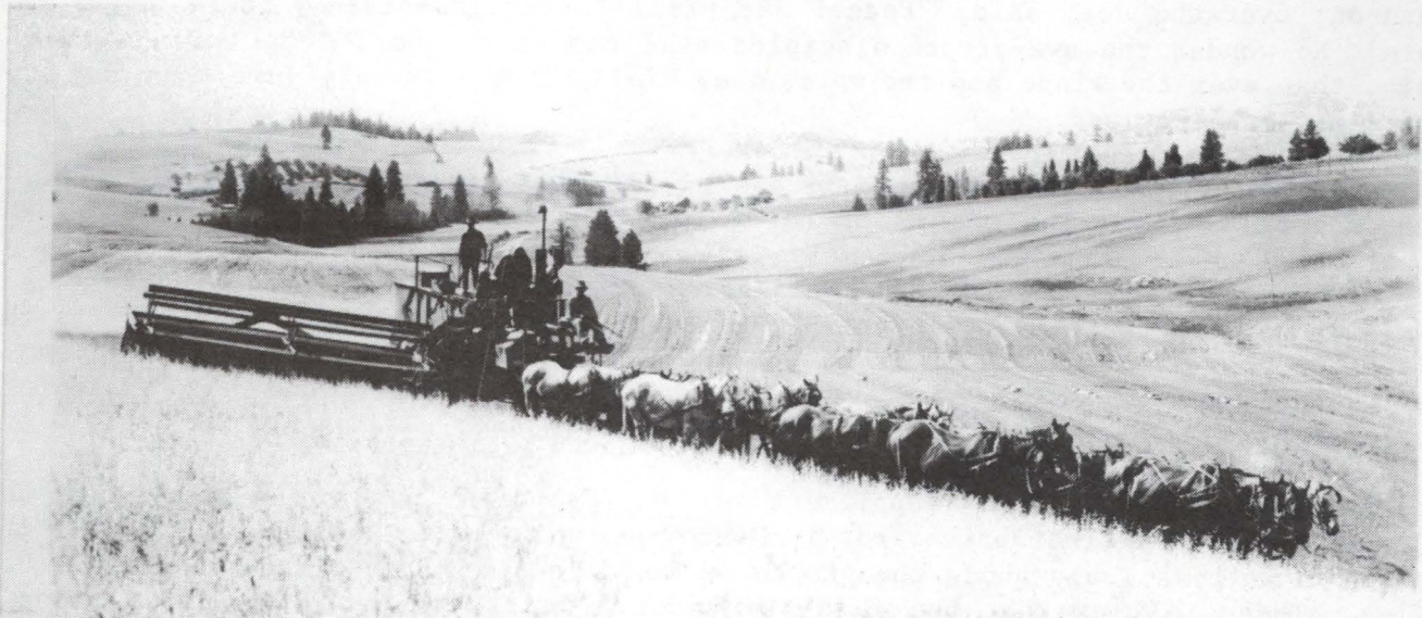
Twenty-seven horse team, 1926. Twenty-seven horses hitched in tandem of four sixes and three leaders are pulling a gas-engine combine in the Palouse hills near Moscow, Idaho. Even though the combine operated with an engine, horses were still needed to pull it over the steep hills.
